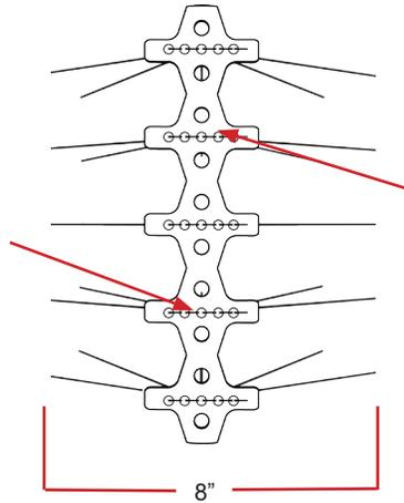
1/4" Screw holes for screw attachment
