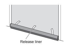
Remove the release liner of the double-sided tape and fix the holder to the door.
