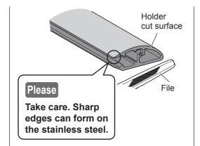
Remove burrs on the holder cut surface with a file.
