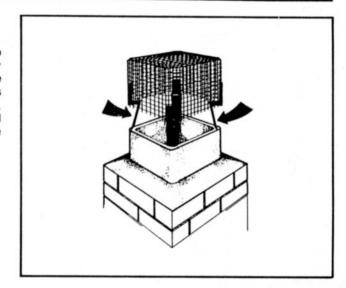
Continue downward pressure until Spark Arrestor/ Screen is completely seated in chimney tile. To remove for chimney cleaning, grasp Spark Arrestor/Screen at opposite corners and gently wiggle it free.
