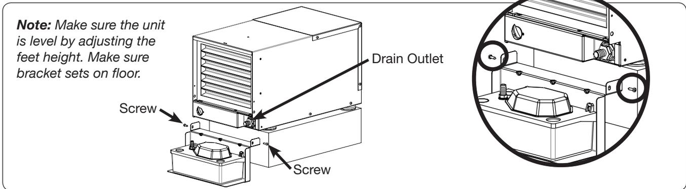
**Step 5.** Attach 5/8" hose onto barbed drain adapter of the dehumidifier. Route hose to condensate pump as shown. Be careful not to kink hose. Trim hose to fit properly. To help with proper drainage, cut hose at 45 degree angle.
