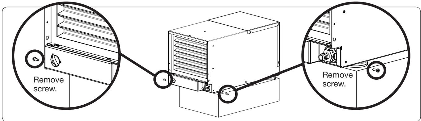
**Step 4.** Attach the condensate pump assembly using the two screws removed in Step 2. Do not over tighten the screws.
