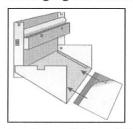
This unit must be used with black glue boards. Simply remove the used glue board from the machine by pulling out of the Uplight cover. For convenience and in locations where the Uplight is mounted close to ceilings etc, the front cover of the unit may be swivelled on the
