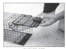
EASY TO SET Simply lift ring on bayonet latch and open door. Move set rod forward so that it supports the door cross bar member and holds the door open.
