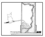
B&G foam application sprayers are used to apply water-based foam to floor drains, wall voids, and enclosed spaces, inside and outside.
