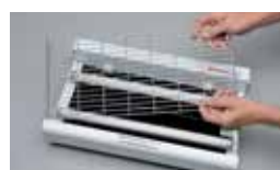
Carefully remove the front grill by slightly bending the tabs at the base of the grill outward from the punched holes and pull away.
