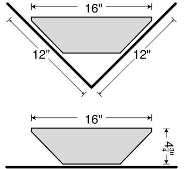
The Junior™, mounts like the rest of the 601 series of traps, in a corner or flat against the wall.
