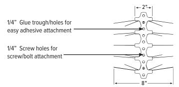
*For Wood:* Use wood screws to secure bird spike strips to wood surfaces. Using pre-drilled holes along the base, screw into the end of each bird spike strip tightly and place one wood screw at least every six inches along the base.
