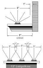
For wide areas, multiple rows of bird spike strips may need to be installed. Install bird spike strips with 1" overlap.
