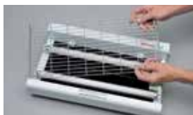
Remove bottom tray and carefully remove the front grill by slightly bending the tabs at the base of the grill outward from the punched holes and pull away.
