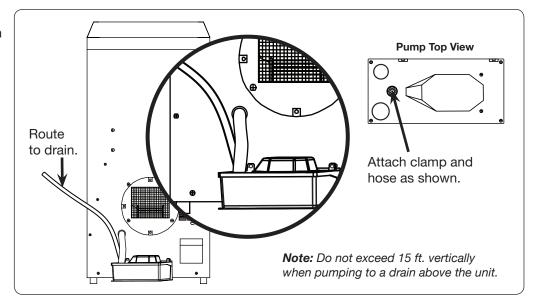
Step 5. Plug the condensate pump and dehumidifier cords into an outlet that is protected with a GFCI device on its circuit.
