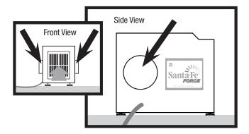
**Step 2:** Before attaching duct collar to dehumidifier, start 6 screws in to pre-drilled holes in the duct collar.
