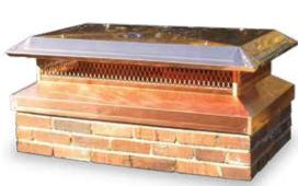
The hood overhangs masonry approximately 1" on both sides and ends. 4¾" skirt protects cement crown from deterioration due to weather. Copper and Stainless Steel are constructed in the same manner.
