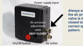
Always ensure that the air pressure valve is tightly closed to ensure correct spray pattern.
