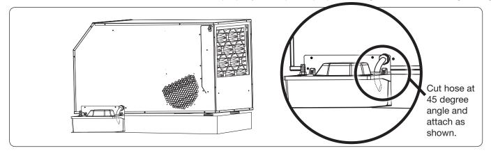
**Step 5.** Insert clamp onto 3/8" drain hose and then attach hose onto the barbed outlet fitting on the condensate pump. Tighten clamp and verify that hose is secured tightly to the condensate pump by pulling gently on hose. Route hose appropriately to a drain.
