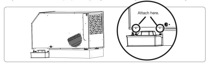
**Step 4.** Attach 5/8" hose onto the barbed drain adaptor of the dehumidifier. Route hose to condensate pump as shown. Be careful not to kink hose. Trim hose to fit properly. To help with proper drainage, cut hose at 45 degree angle.
