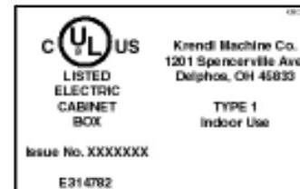
Indicates that the electrical box on the machine is in compliance with UL codes.
